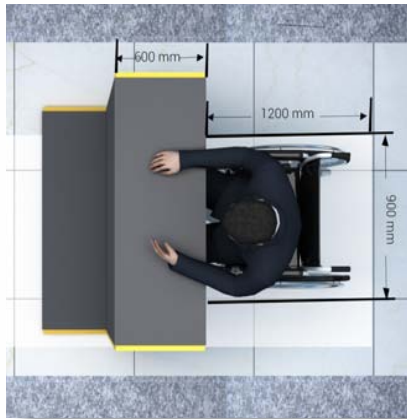
Figure 60 - Clear Floor Space for wheelchair
