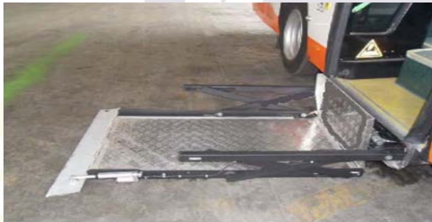
Figure 117 - Platform Installed Under Step of Bus
