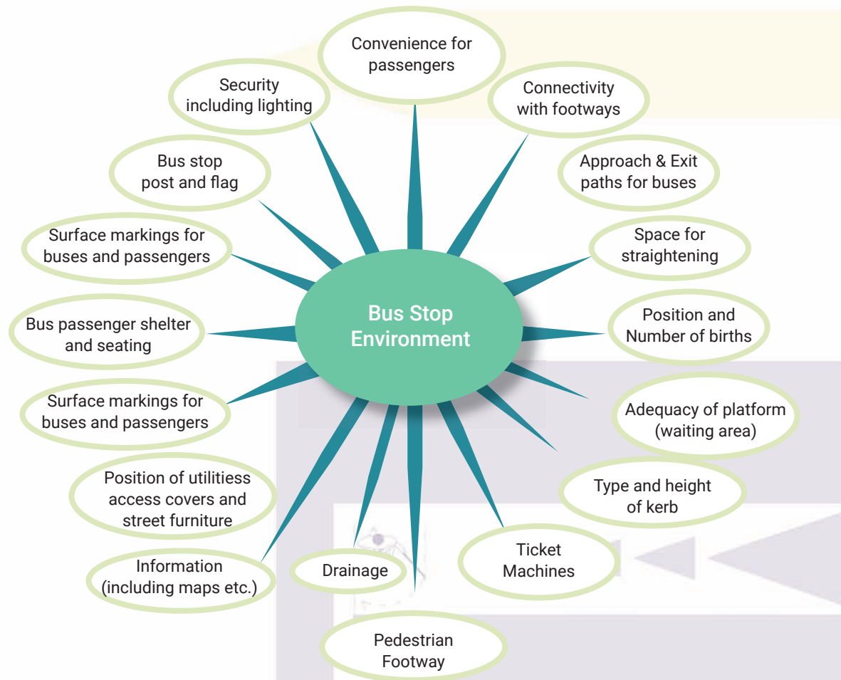
Figure 104 - Bus Stop Environment
