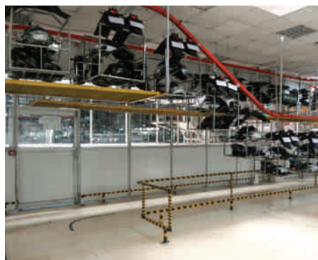
FG Over Head Conveyor
