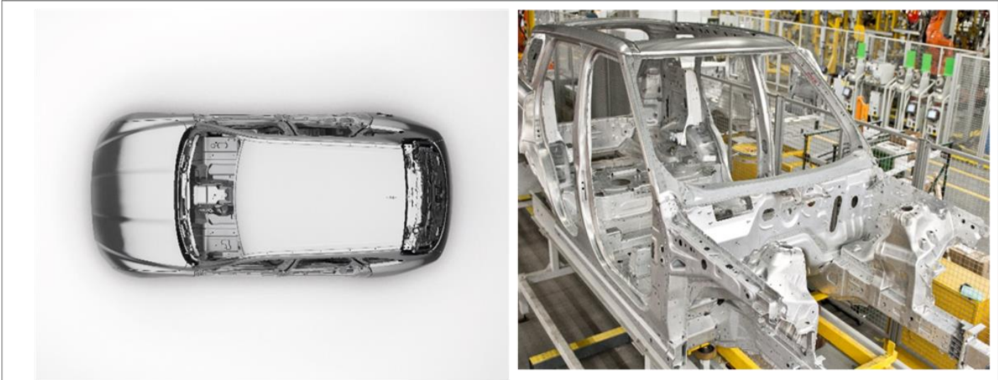
Figure 11: Vehicle monocoque chassis frames of Jaguar F PACE (L) and Range Rover
