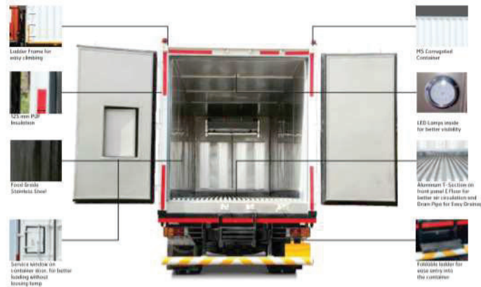
General Arrangement of a Reefer van
