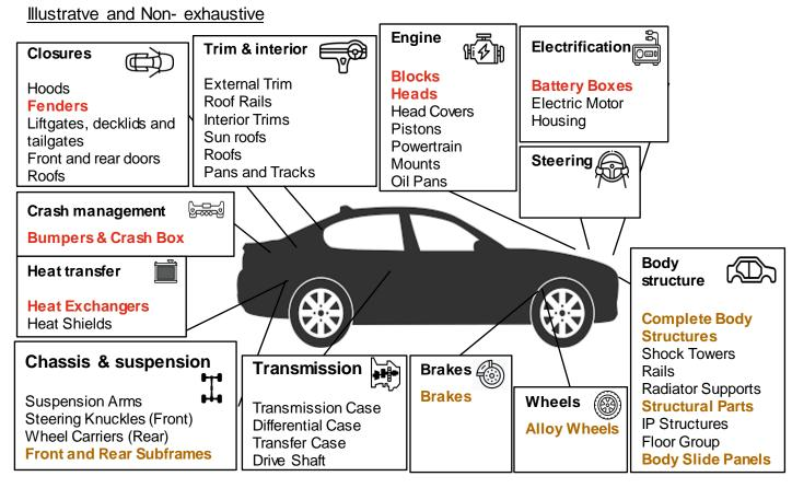
Note: The components of the car above encompasses all aluminium applications in a European passenger car and is based on the analysis of a car sample covering nearly 95% of total EU28 production
